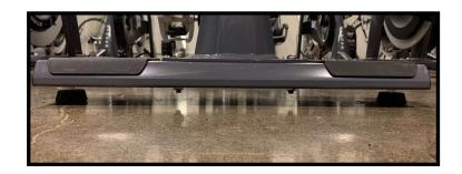
To begin you will need to level the bike. Make sure the front two leveler feet on the front stabilizer are screwed all the way up to the frame, even and level. On the rear stabilizer, screw the leveler feet all the way up to the frame then only adjust the left or right rear leveler feet to level the bike. In some cases just by leveling the bike, the vibration or rough ride could go away and no adjustment on the flywheel would be needed.
