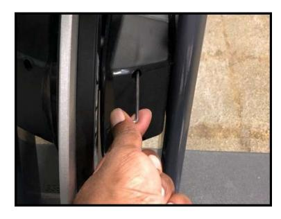
Remove the two bolts on both front covers with a 3mm allen.
