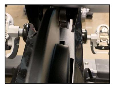
Ride the bike and press down the brake to make sure the flywheel is not rubbing on the magnets. If flywheel is rubbing on the magnets, adjust the magnets away from the flywheel.
