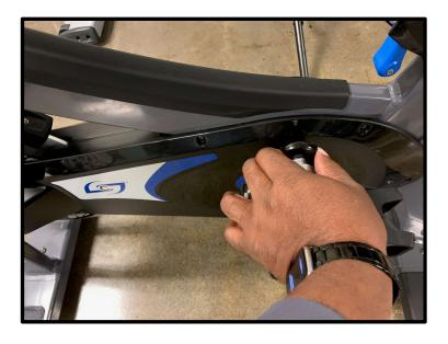
Check the belt tension (deflection) on the bike. Position the crank in the 12 o'clock position then press down the resistance knob to hold the crank in place. Grab the crank with your hand and move the crank forward and back while continuing to press down the resistance knob. There can be up to a 1/8 of inch of deflection in the crank. Follow the next steps to adjust the deflection.
