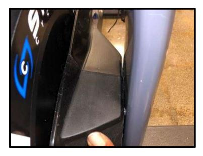
Install the left and right front covers back on the bike. Make sure that both of the front covers line up with seam of side covers and then tighten the bolts with a 3mm Allen key.
