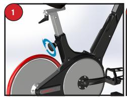
Turn the Adjustment Knob approx. 1/4 to 1/2 turn counter-clockwise until it loosens.
