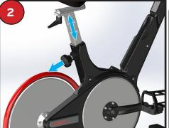
Pull the Adjustment Knob out towards Re-engage the Adjustment Knob, you. While holding the Adjustment ensuring it locks into the desired hole Knob, raise or lower the Seat/ in the Seat/Handlebar Post. Turn the Handlebar Post to reach the desired knob clockwise until it is hand tight. position.
