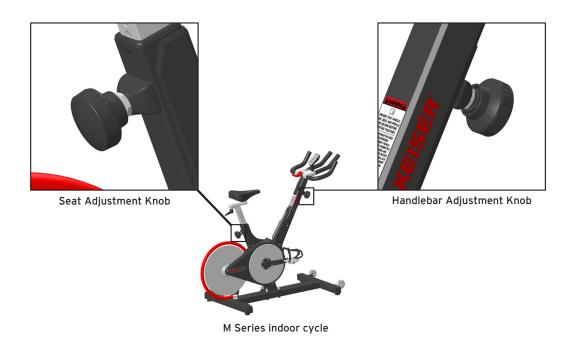
WARNING: Always check Adjustment Knobs before exercise to ensure they are locked and tightened. Failure to follow seat/handlebar adjustment procedure may potentially result in personal injury and/or property damage. Ensure instructions are read and understood before exercise or seek help before use.
