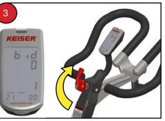
Set shift lever to gear 21 for Miles, or set shift lever to gear 19 for Kilometers.
