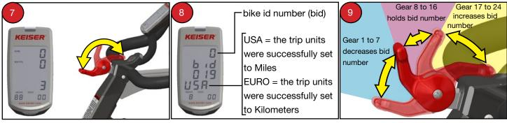
Move the shift lever from stop to stop 6 times.
