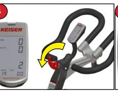
Set shift lever to gear 19 for Miles, or set shift lever to gear 21 for Kilometers.
