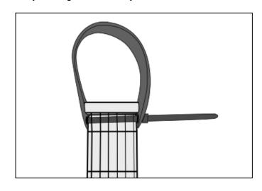
Feed the cable tie through the left back side of the leather Traveler Guitar strap.
