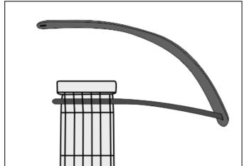
With the guitar strings facing up, slide the cable tie under the strings and behind the nut starting from the right side of the neck. Pull the cable tie all the way through until it stops at the cable tie lock.
