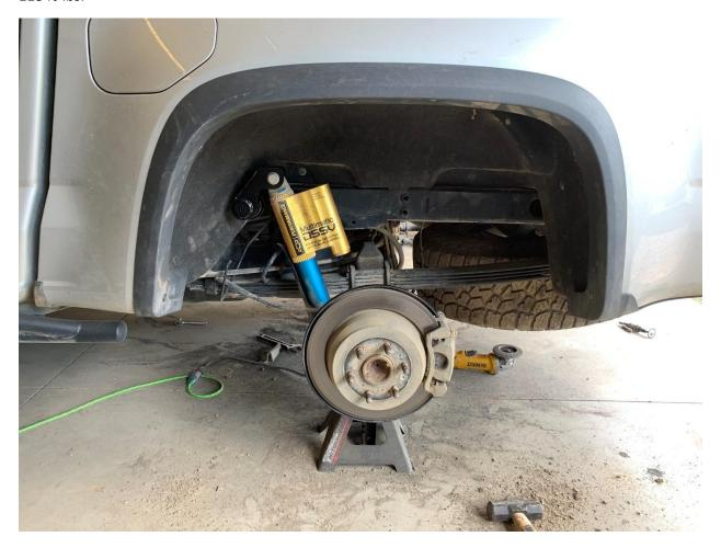
**Step 10:** Reinstall the rear tires. Lower the vehicle off of the jack stands and torque lug nuts to factory specifications.
