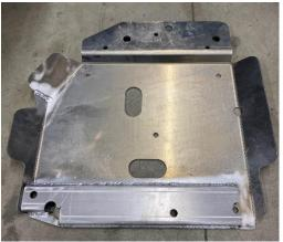
**Step 5:** Locate the Oil Pan skid plate and (3) M10x1.5 bolts. While supporting the transmission skid, remove the previously installed (2) M10x1.5 bolts near the engines oil pan. Bring the Oil Pan skid into position and loosely re-install the (2) M10x1.5 bolts, sandwiching the transmission skid between the crossmember. Install (1) M10x1.5 bolt into the front of the oil pan skid to temporarily hold it in position.
