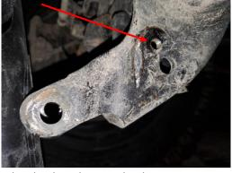
**Step 4:** Compress the shock and move shock in to position within the factory mount and shock skid. Use the included longer bolt to feed through. Reuse the factory nut. (Pictured to the left)
