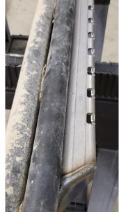
**Off-roading:** If doing heavy rock crawling where slider interaction with rocks could be frequently, it is recommended to remove the Slider Steps.
