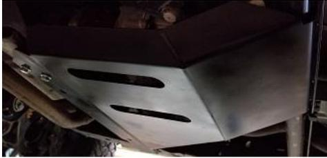
**Step 3:** Place the skid into place and insert all 4 bolts (15mm socket), including the rivnut on tab through the side of the crossmember and tighten (as shown on first page).
