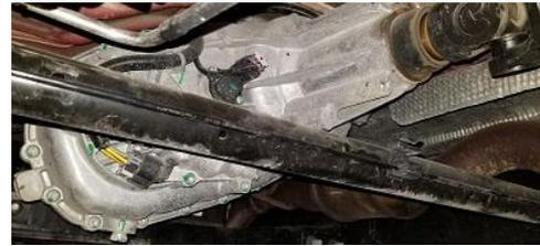
**Step 4:** Mark a point to drill, or begin with a smaller pilot hole in the center of the hole. Drill to 9/16". Repeat for both holes.
