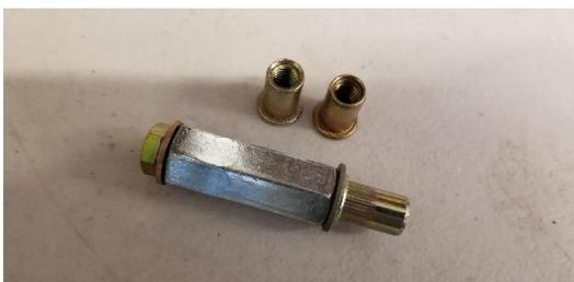
**Step 4:** If you're not installing the additional rivnuts, skip to the **Step 6**. If you are installing the additional rivnuts, [here is a short video to explain how to use the rivnut tool](#). First you will need to drill the 2 holes. Line up the mount with the existing bed holes and mark where you will need to drill. Use a 7/16" drill bit to drill your 2 holes.
