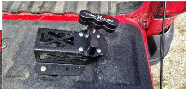
**Step 2:** Attach the Rotopax and determine which position in the bed you would like to use. Remove the Rotopax once you have determined the location you'd like the mount. There are 4 different locations in the bed: front left, front right, left rear, and right rear.
