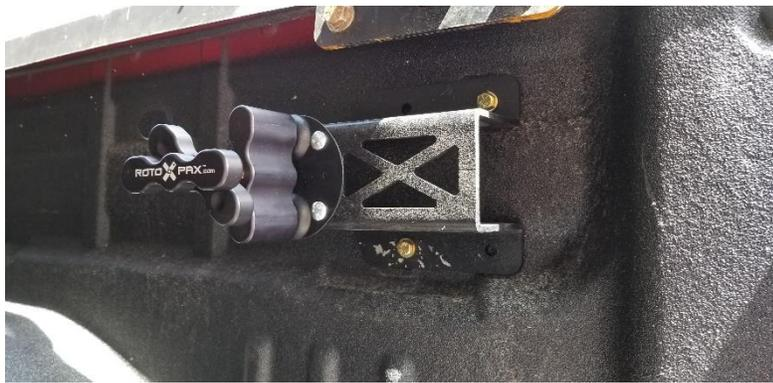
**Step 7:** Position the tabs so that the long side will slide into each of the holes first. It **IS** a tight fit, but it helps the mount be very rigid with the bed side. Once they are in, tighten with the 1/2" socket. If additional rivnuts were used, install that hardware as well.
