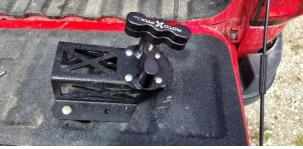
**Step 2:** Attach the Rotopax and determine which position in the bed you would like to use. Remove the Rotopax once you have determined the location you'd like the mount. There are 4 different locations in the bed: front left, front right, left rear, and right rear.
