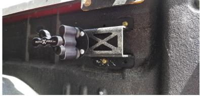
**Step 7:** Position the tabs so that the long side will slide into each of the holes first. It <u>IS</u> a tight fit, but it helps the mount be very rigid with the bed side. Once they are in, tighten with the 1/2" socket. If additional rivnuts were used, install that hardware as well.
