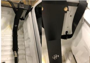
**Step 4:** Make sure you clip the large ratchet strap into the carrier before bolting it down and run the lashing strap through the tie down hook. Then tighten the 4 bolts in the bed and the clamp on the bed side.
