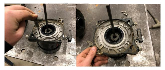
**Step 4:** Reassemble the gearbox to the winch drum and support rods. Align the drive shaft with the other half as you slide the winch back together. (Note: the clutch lever will now be on the bottom) Reinstall the two large screws into the support rods.
