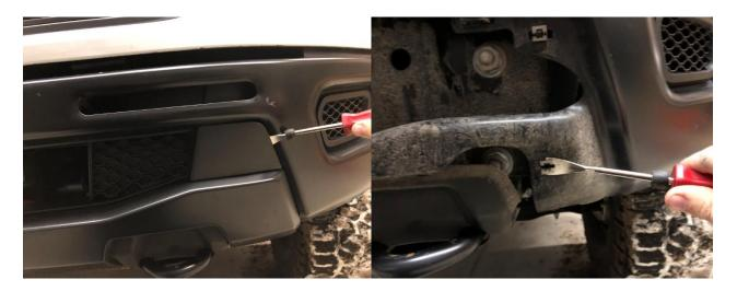
**Step 3:** With the plastic insert removed, you can now un bolt the steel bumper. Start by removing the six 21mm nuts. With the nuts removed and the bumper loose, unplug the factory fog lights if equipped. Set the bumper aside out of the way.
