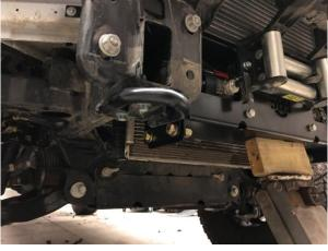
**Step 6:** Loosely install the factory tow hooks and fasteners, sandwiching the bracket between the frame. The tow hooks have a small locating tab that will need to bent out of the way or removed. The attached skid plate mount will not need to be touched, unless install aftermarket skid plates. You may need to raise the mount with a jack to get the brackets close enough to the frame.
