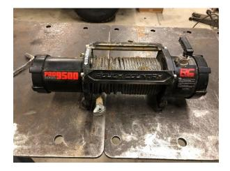
**Step 2:** On the side of the winch with the clutch release lever, remove the two large screws holding the gear box to the support rods. (this allows you to separate the gear box from the winch drum.) With the screws removed, you can separate the halves.
