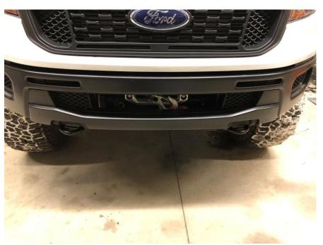
With all the fasteners removed, you can start carefully prying the plastic insert by starting on the drivers side with a trim tool, and working your way to the passenger side. Note: the metal clips may stay in the steel portion of the bumper. Remove these and re-attach to the tabs on the plastic insert.
