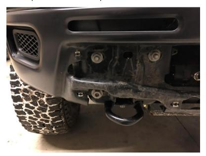
**Step 4:** Remove all plastic shrouding and associated mounts to expose the radiator and make room for the winch. Remove the factory tow hooks now using the 15mm socket and ratchet. Save for reinstall later.
