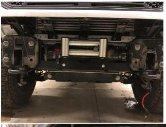
**Step 8:** Route the winch wiring up to the engine compartment. The battery is on the driver's side. Be mindful of moving parts and wires chaffing on metal components.
