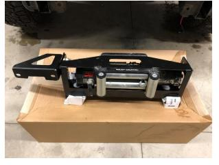
**Step 3:** Now is the time to wire the winch. The control box will now be mounted under the hood. You will need longer leads to wire it (Not included). Be sure to use the same gauge wire that is supplied with your winch.
