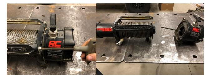
**Step 3:** With the clutch side of the winch removed. Remove the series of small screws that attach the mounting block to the gear box. With it removed, rotate the mounting block 180 degrees and reattach. The mounting feet should now be on the same side as the clutch lever. Use caution when tightening the small screws. DO NOT OVER TIGHTEN, but make sure they are snug.
