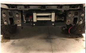
**Step 5:** Loosely install the lower brackets to the winch mount with the supplied ½ inch bolts, lock nuts and washers.
