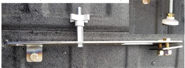
Step 1: After determining which side of the bed you would like your jack mount located, pinch the top of the bed rail under the plastic rail and attach the bottom mount to the bed loop as seen in the pictures to the right. Tighten bolts to secure the mount.
