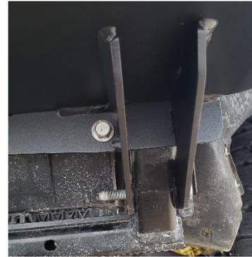
**Step 12:** Trim and reattach the inner fender liners. You may need to secure the forward inside part of the liner as it is now not attached.
