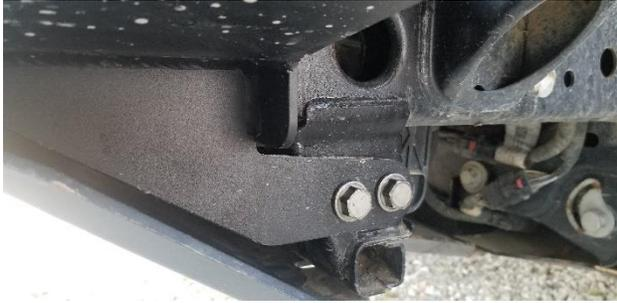
**Step 11:** Reinstall all the remaining fasteners into the fascia, and installing the bumper using factory crash bar and tow hook hardware. Be sure to install your desired winch into the bumper, and plumb the wiring before installing the bumper.
