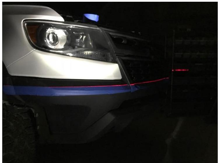
**Step 8:** With the factory fascia reinstalled, take the blue painters tape and follow the laser line across the fascia. Keep the pieces of tape small in length (6-8") to help make it easier to follow the line.
