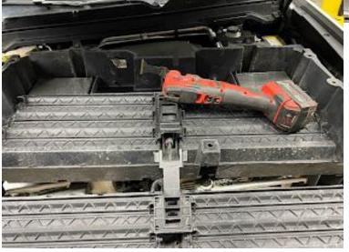
If equipped with active shutters, you will need to remove the plastic arm connecting the upper and lower shutters. One you have trimmed the shutter housing, you can reinstall it.
