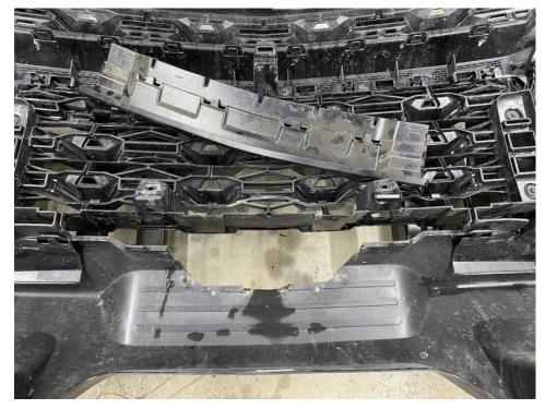
**Step 3:** Now we can measure for trimming the fascia to install the receiver close out panel. Located the tabs in the center of the lower portion of the fascia. Measure in, towards the center, 1 ¼ inches from both tabs and make a mark with your sharpie.
