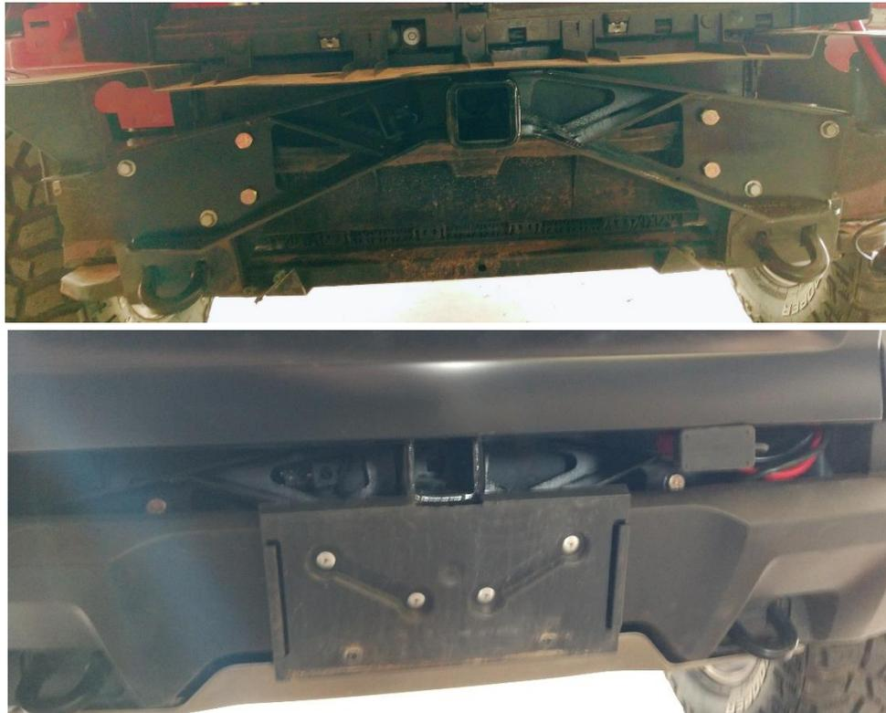
**Notes:** Minor trimming of the fascia may be required around the receiver. Relocation of the outdoor temperature sensor may be required.
