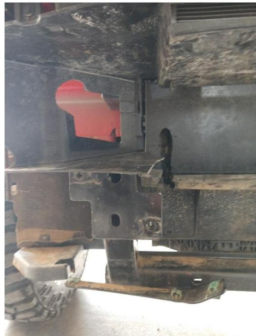
**Step 3:** With the fascia removed, remove the crash bar that's bolted to the front of the frame rails, using the 15mm socket. Next, remove the factory tow hooks and hardware with the 18mm socket and wrench.
