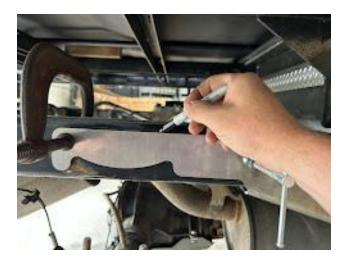
**Step 5:** With the bracket traced out on the frame, you can remove the paint along the line to prep for welding. Since the frame is fairly thin to start with, we recommend using a wire brush to remove any paint and not make the frame thinner from grinding. Using some heat from a propane torch can help soften the paint for easier removal. (Be aware of your surroundings when using an open flame)
