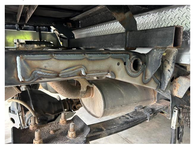
**Step 9:** With the bracket fully welded and cooled, prep and paint any bare metal with a heavy duty paint.
