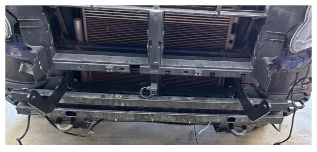
Step 5: To reinstall the air dam, you will need to trim the sides off, so it can fit between the frame brackets. Reinstall all push clips after trimming. \* Now is a good time to run the wiring for your lights.
