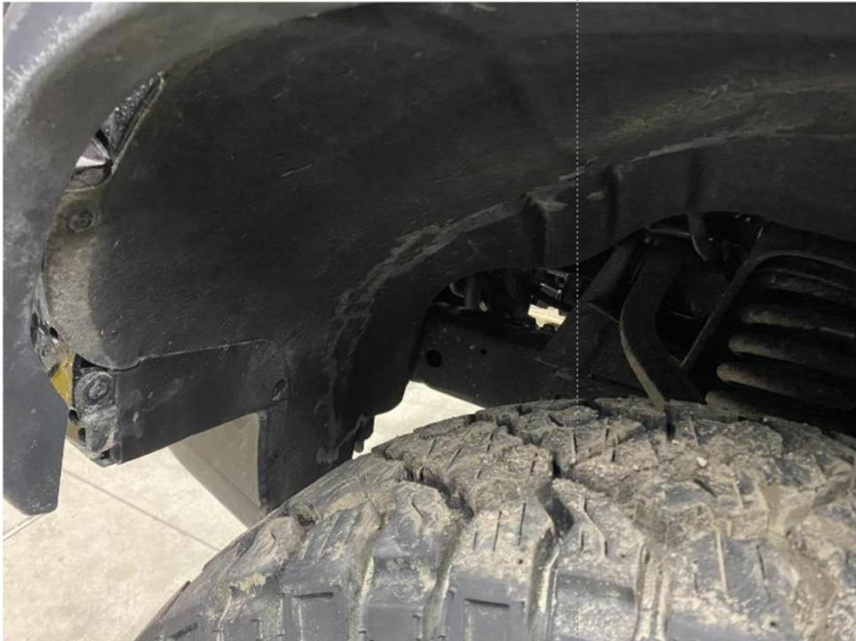
**Step 3:** With the fascia removed, You can start by removing the plastic air dam above the crash bar. There are three push clips on the top and a clip on either side, along with two clips between the push clips. Use a small flat head screwdriver to release these. Next you remove the two crash bar bolts, on one side, using the 15mm socket and ratchet.
