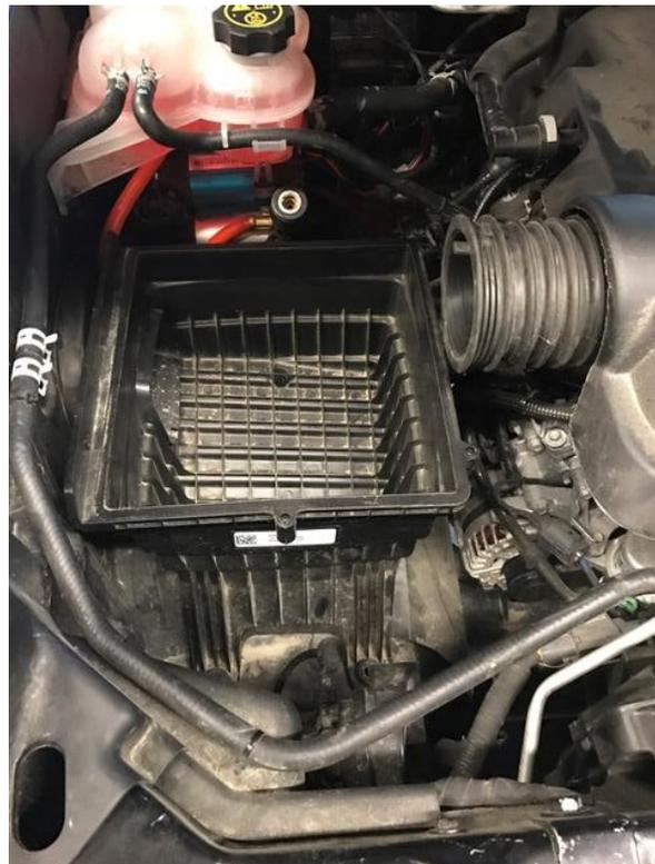
**Step 2:** With the air box out of the way, you now remove the two 10 mm nuts holding the reservoir tank to the vehicle. The reservoir will be able to lift up off the studs and you can roll it out of the way. Be cautious as the tank can be hot if the vehicle was running recently. It can also leak out of the cap.
