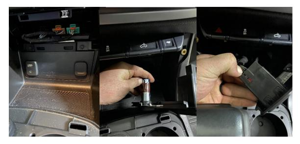
**Step 5:** Remove the USB and Cigarette lighter sockets from the plastic panel and simply clip them into the Command Center panel. If you have heated seats, install those buttons into the Command Center at this time, also.
