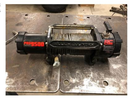
**Step 2:** On the side of the winch with the clutch release lever, remove the two large screws holding the gear box to the support rods. (this allows you to separate the gear box from the winch drum.) With the screws removed, you can separate the halves.
