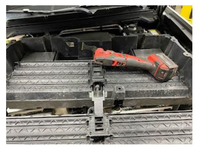
Step 4: Remove the crash bar that's bolted to the front of the frame rails, using the 15mm socket.
