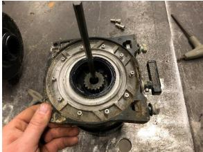
**Step 4:** Reassemble the gearbox to the winch drum and support rods. Align the drive shaft with the other half as you slide the winch back together. (Note: the clutch lever will now be on the bottom) Reinstall the two large screws into the support rods.
