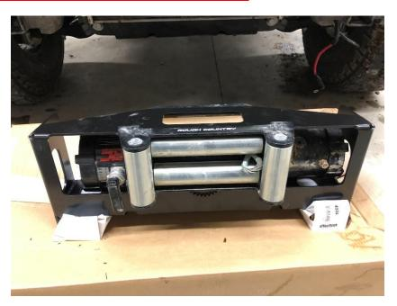
Step 2: Flip the mount up and install the winch fairlead into the upper winch mount holes. Be sure the bolts you are using are proper length to fit through the fairlead and have enough engagement into the winch.
