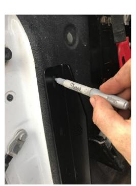
**Step 2:** Starting on the drivers side. Place the bracket into position and check clearance with the tailgate
