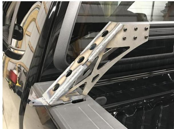
**Step 4:** With the whole bed bar kit loosely assembled, with a partner, lift the assembly and slide it into the bed pockets. Loosely install the supplied ½" hardware, into the existing hole in the inner bed side, to attach the bed bar bracket to the bed.
