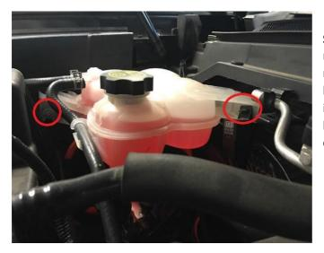
**Step 2:** With the air box out of the way, you now remove the two 10 mm nuts holding the reservoir tank to the vehicle. The reservoir will be able to lift up off the studs and you can roll it out of the way. Be cautious as the tank can be hot if the vehicle was running recently. It can also leak out of the overflow.
