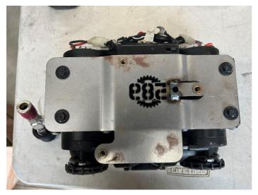
**Step 4:** Mount the air compressor to the bracket using the supplied hardware with the compressor. The filter side of the compressor will be on the bottom side of the logo.
