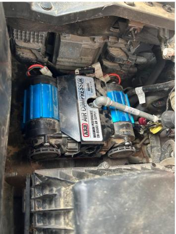
**Step 5:** Lower the compressor and mount into the engine bay, onto the inner fender. Align the holes and install the two rear most bolts, that are included with the mount. Loosely install the third bolt, and fully tighten the rear most bolts. Remove the loosely installed bolt, pull the fender liner back into position, and reinstall the third bolt through the liner and tighten. Reinstall the T15 screws and fender flare.
