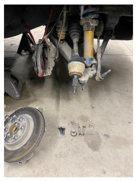
**Step 7:** With the upper control arm removed from the steering knuckle, you can now remove the 36mm axle nut and washer. Next remove the lower ball joint nut using the 26mm socket and ratchet. A few light taps on the steering knuckle should release it from the lower ball joint. You can know slide it off the spines of the CV axle and place to the side.
