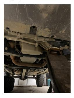
**Step 12:** With the differential supported by the jack, you can now remove the front differential brackets on each side using the 21mm socket and 15mm socket. You will reuse the 21mm head bolts, however, the 15mm head bolts along with the factory brackets won't be reused.
