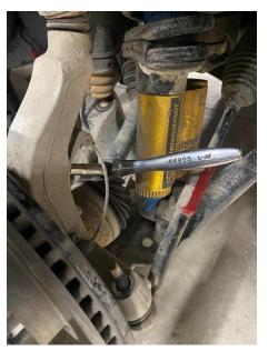
**Step 5**: Remove the T30 torx screw from the wheel speed sensor, along with the 10mm head bolt holding the wheel speed sensor wire. The speed sensor can be gently removed from the steering knuckle and moved out of the way. Also remove the outer tie rod end using the 21mm socket and ratchet.
