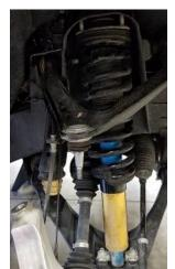
**Step 2:** Remove the two lower strut bolts from the lower arm with a 15mm socket and ratchet. Using a 13mm socket and 15mm wrench, remove sway bar links.
