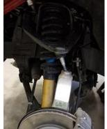
**Step 7:** Remove the factory bump stop, and insert the new extended bump stop. They can be a nice snug fit and need a little force to fully seat.
