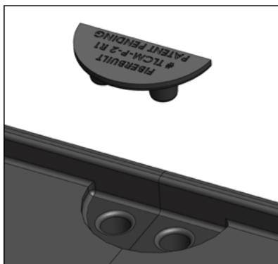
2-Pin Connectors (H) for side connections
