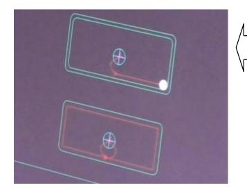
FOR 30mm MATERIAL (*OR THICKER*) THE DIMENSIONS AND THE 20mm DEEP REBATE REQUIRED ARE ENTERED INTO A COMPUTER CONTROLLED ROUTER MACHINE . . .
