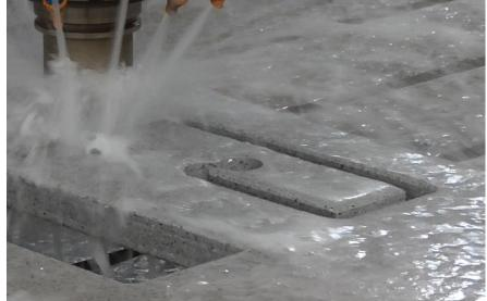
THE TOOL THEN RETURNS TO THE WORKTOP TO CARRY OUT ITS SECOND GRINDING PROCESS AND CREATES THE REBATE (at -20mm DEPTH) FOR THE S-BOX<sup>™</sup> COLLAR TO SIT ON LATER.
