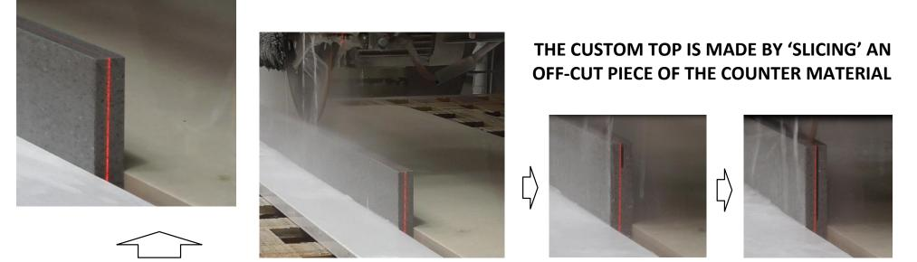
THE CIRCULAR SAW FOLLOWS A LASER LINE, AND CAREFULLY CUTS THE THICK MATERIAL DOWN INTO THE 12mm THICKNESS REQUIRED. THIS IS DONE IN A SERIES OF 8-10 PASSES TO ENSURE THE INTEGRITY OF THE STONE.
