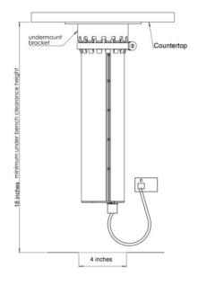
Colour: Clear and Black anodized aluminium Material: Polvamide and ABS Hole size: 101.6 mm Inner disc size: 93mm Required space: 450mm depth Package size: 65mm x 19mm x 13mm Weight: 2.kg Cable length: 1.7 m Socket configuration: 2x power outlets 1 x USB -A & 1 x USB -C Supply Voltage: 125V ac 60Hz Max Current: 15a Ingress rating: IP44 Designed and engineered in Australia. Made in Vietnam
