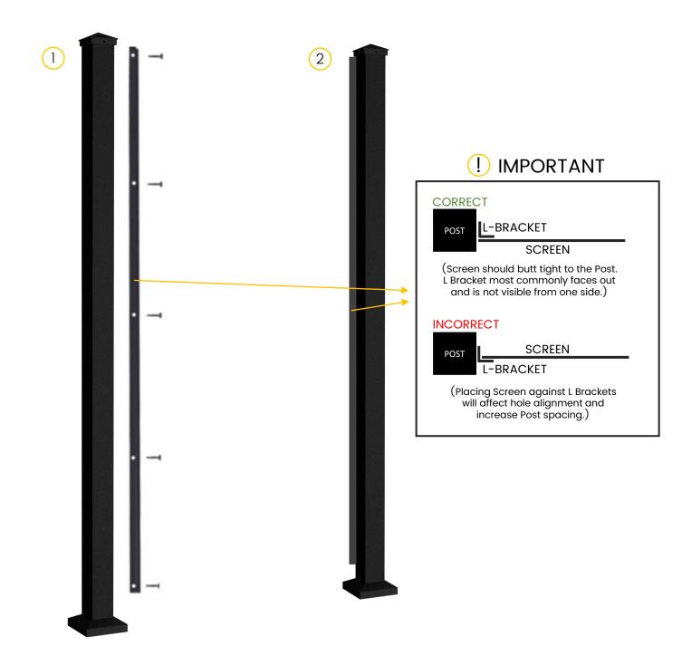
Butt L Brackets against the bottom edge of Pillar Caps and the center of each Post. Fasten (5) self-tapping screws through L Brackets and into each Post.. (an awl or 1/8" metal drill bit can be used to drill pilot hole in L Bracket. We recommend drilling about ½" below the factory hole on
