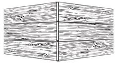
**BUTT CORNER (right drawing)** - the panels can simply be butt together to create a finished corner.
