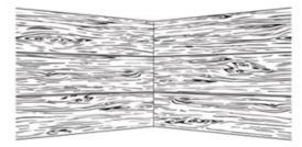
**BUTT CORNER** - Butt two panels together at the inside corner. If there are any unwanted gaps, the paintable caulking and BARN**WOOD** Paint Kit can be used.
