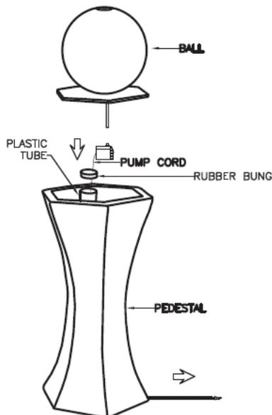
2. Fill reservoir with appropriate amount of water to fully submerge the pump.
