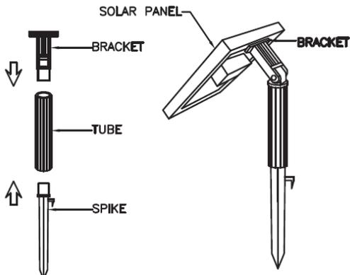
6. Insert the spike into the ground. Position the solar panel so it's facing south (in northern hemisphere) as much as possible to maximize daylight hours. It is important to angle the solar panel to face the sun when the sun is at its highest point. Ensure the solar panel is not shaded by trees, shrubs or buildings.
