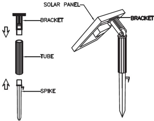
5. Insert the spike into the ground. Position the solar panel so it's facing south (in northern hemisphere) as much as possible to maximize daylight hours. It is important to angle the solar panel to face the sun when the sun is at its highest point. Ensure the solar panel is not shaded by trees, shrubs or buildings.
