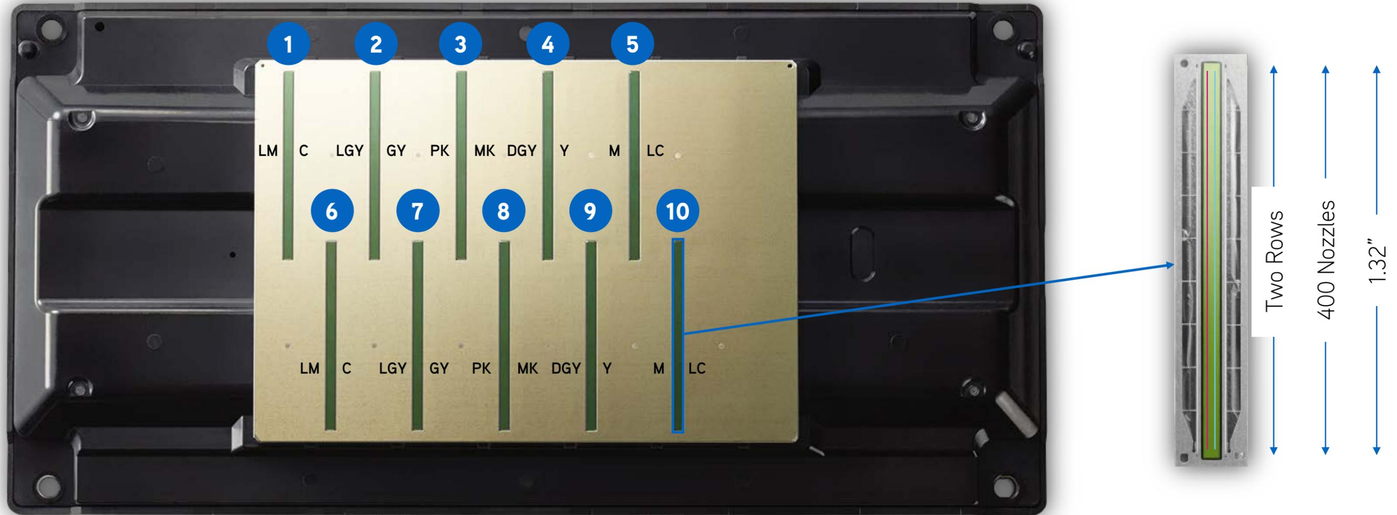
The PrecisionCore MicroTFP printhead is developed using 10 individual PrecisionCore “blades”. Each “blade” has two rows - one for each color - using 400 nozzles each across a 1.32” width. When combined, the final printhead array prints using 800 nozzles per color over a 2.64” print width.
