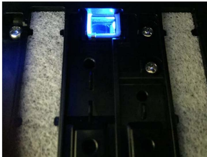
**Actual CMOS sensor photographs the back-side of the media in realtime to help determine media movement.**
