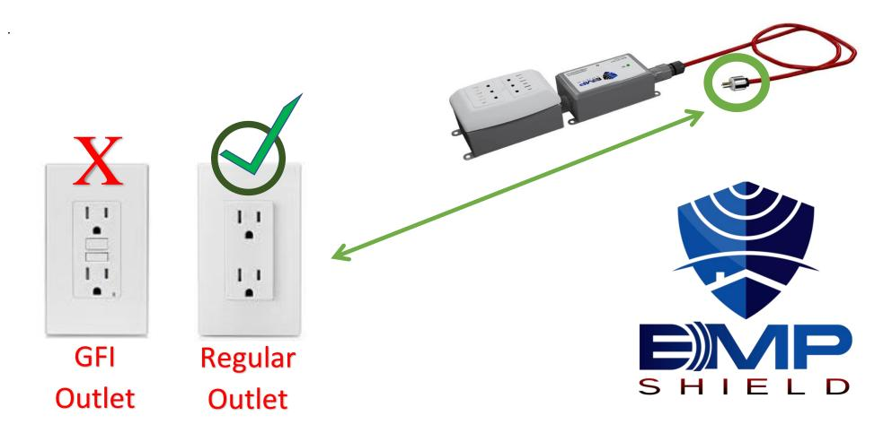
Plug-in the EMP Shield into a Non-GFI outlet and the entire 110V electrical phase will be protected.
