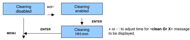
The activation of **compulsory cleaning** function is made with + or - keys.
