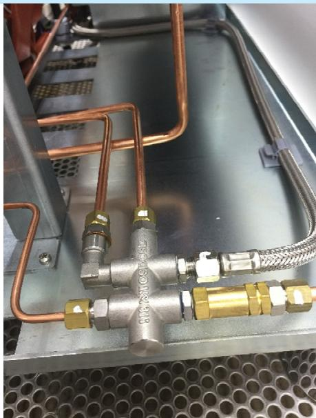
*This part, placed in the right side, under the boiler is a special fitting that distributes the cold water to the steam boiler, the coffee groups, the heat-exchanger and the mixer of the hot water dispenser.*
