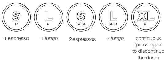
To program the amount of coffee, with the machine on and ready to make coffee (keys of the keypad permanently lit), press the programming button XL for 5 or 6 seconds until it is lit intermittently while the rest of the keys are illuminated in a fixed manner.
