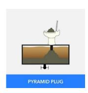
Compacted Tank – solid waste accumulated in the bottom of your black tank, preventing waste from exiting when the valve is opened. Reasons include:
