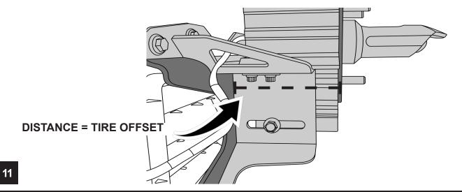
TORQUE THE SET BOLTS AND INSTALL THE SPARE TIRE AND TORQUE TO 90 FT-LBS
