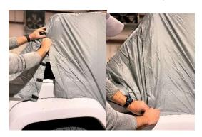
At front tire on both sides of vehicle secure hooks in vehicle chassis and tighten straps. (Same for 2 door versions)
