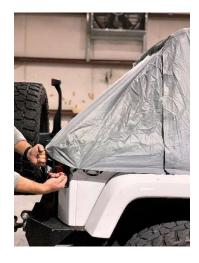
Attach strap around spare tire. Buckle and secure. (Same for 2 door versions)
