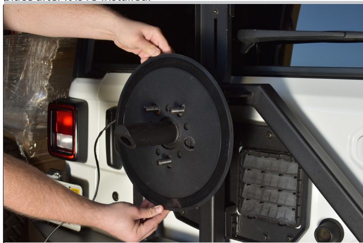
PIC 01: Remove the OE hinge bolts.
