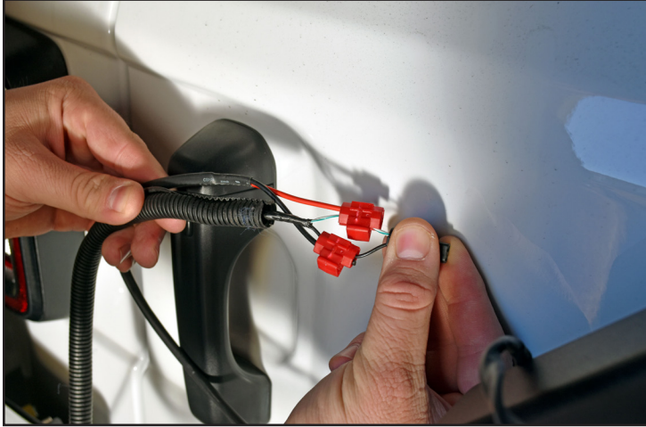
PIC 01: Make the electrical connections.
