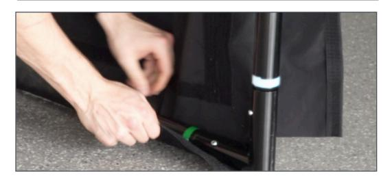
Now, with the black surround atop the frame, you can attach it to the frame by pressing the velcro flaps around the poles. Once securely fastened to the frame locate
