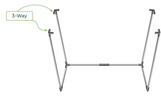
Note: Do not over-tighten set screws with force. Tighten enough so that you feel or hear slight click.
