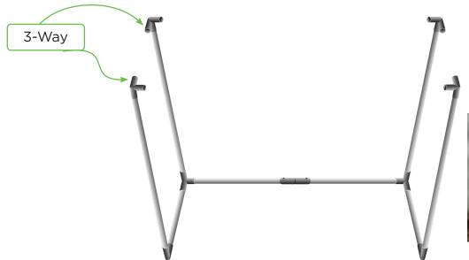
Note: Do not over-tighten set screws with force. Tighten enough so that you feel or hear slight click.
