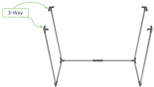
Note: Do not over-tighten set screws with force. Tighten enough so that you feel or hear slight click.
