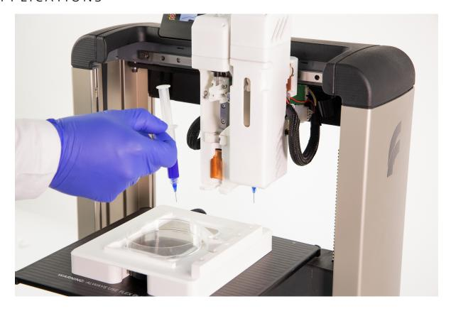
The printer is characterised by key features that are specifically designed for medical, scientific, and research applications, including syringe cooling / heating, print bed cooling and heating, a dual head system, easy syringe positioning (ergonomic access to the machine supports researchers in their work), and automatic bed levelling.
