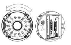
Close properly the battery compart and replace the front cover, making sure correct position of the cable to avoid compromising their integrity and functionality of the unit control. After power-on, all LED lights turn on for 1 second and then go out. After the light is off, follow-up operation can be carried out.
