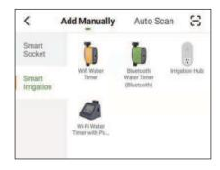
② Follow the app setup wizard. Press and hold the button on your timer around 5 seconds until the blue LED light rapidly flash. Then, press to confirm on your app.
