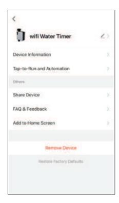
Press the pen selection on the top right corner of the parameter page. There are basic information like Device Information, Tap-to-Run and Automation and other basic functions and services for the device.
